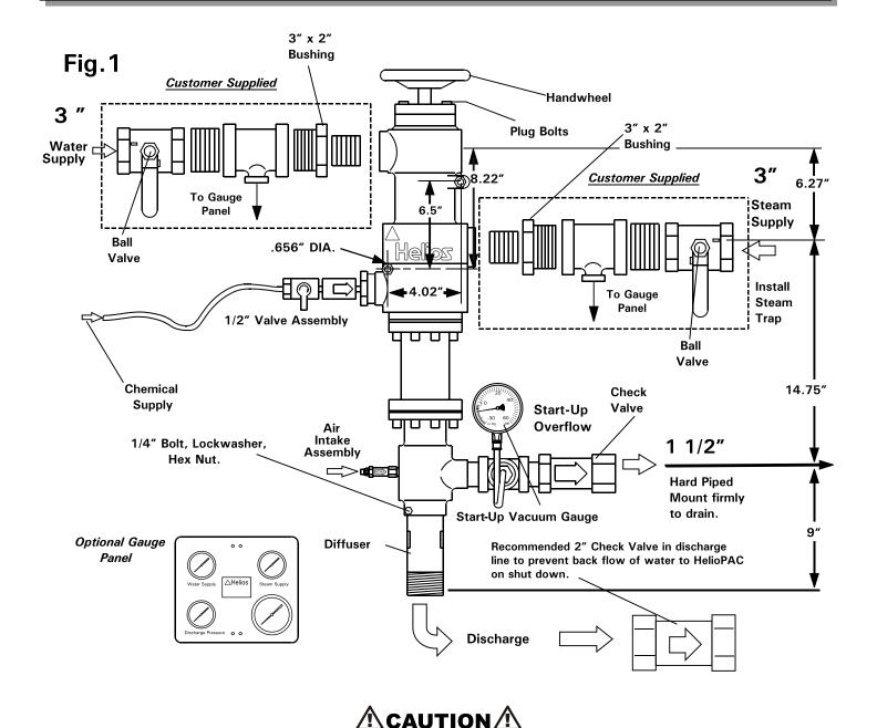
The HelioPAC **MUST** be installed strictly in accordance with the installation requirements of Fig. 1. Follow **ALL** local codes.
